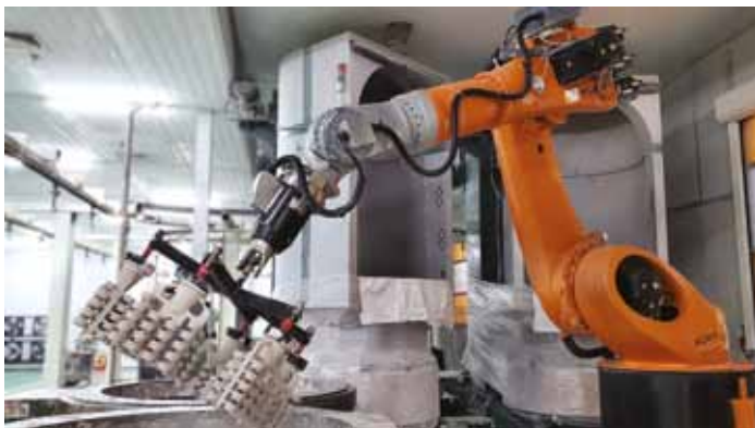
Automation production line – shell moulds system.
